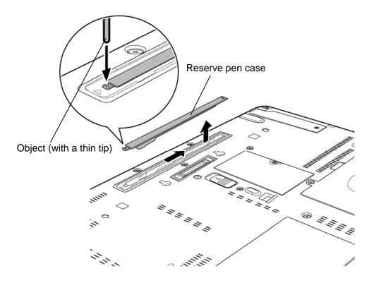
Figure 4-5 Removing the reserve pen case
